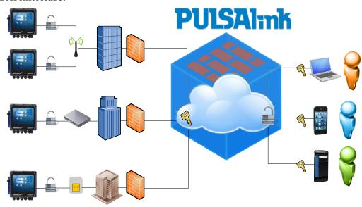
Access your controller securely through PULSAlink. Encrypted two way communication. Leave networks protected and secure without the need for any modifications.
