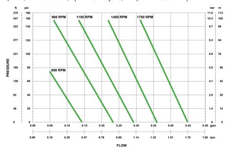
Actual performance to be within +/- 6% for total head and +/- 8% for rate of flow for any given position on the published performance chart
