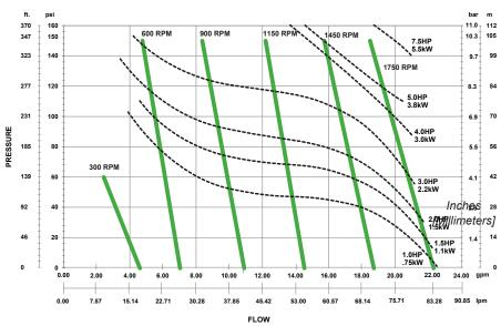
Actual performance to be within +/- 6% for total head and +/- 8% for rate of flow for any given position on the published performance chart
