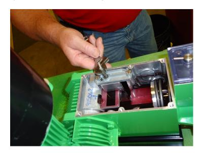
Adjust the shaft to the zero stroke position.
